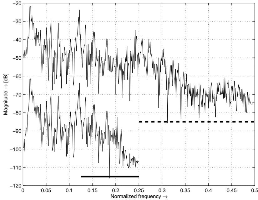
Figure 10: Input and bandwidth extended spectra. The horizontal lines indicate the passbands of FIL1 and FIL2. The input spectrum is offset by 40 dB.
