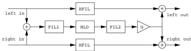
Figure 1: *Signal processing for psychoacoustic bass enhancement. The input signal is summed and filtered to obtain the bass portion. Then harmonics are created and added to left and right output signals. In the direct path a high-pass filter is implemented.*
