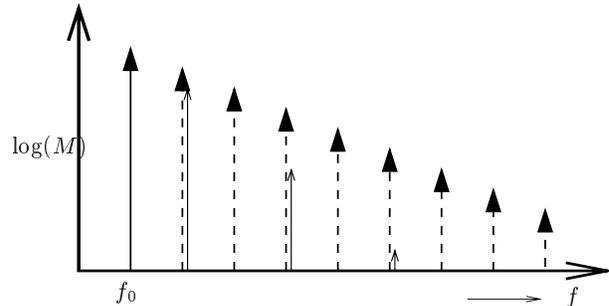
Figure 5: The solid arrow at  $f_0$  represents the input spectrum. The arrows at  $2f_0$ ,  $4f_0$ , etc., represent the output spectrum for the full wave rectifier, the dashed arrows at  $2f_0$ ,  $3f_0$ , etc., represent the output spectrum for the full wave integrator.
