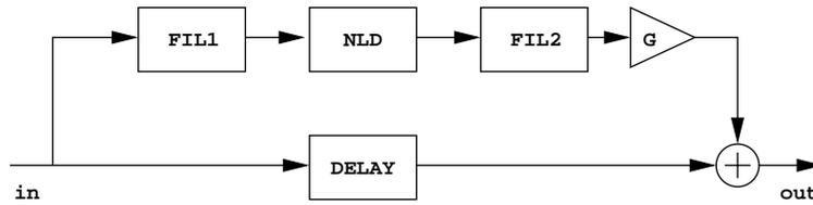
Figure 8: High-frequency bandwidth extension.
