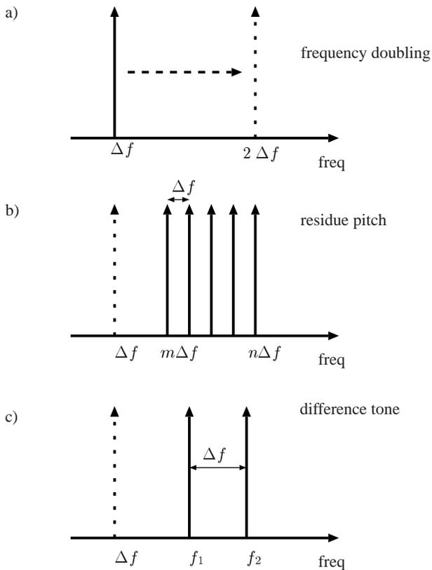
Figure 2: Possible options for psychoacoustic bass enhancement. The dotted frequency component denotes the perceived pitch (but is not necessarily acoustically radiated).
