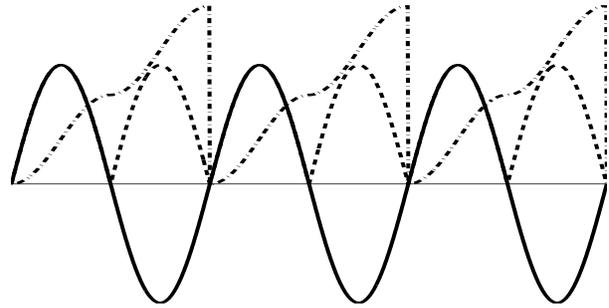
Figure 4: The solid line represents a sine wave input. The dashed line is obtained by full wave rectification, the dash-dotted line by full wave integration.
