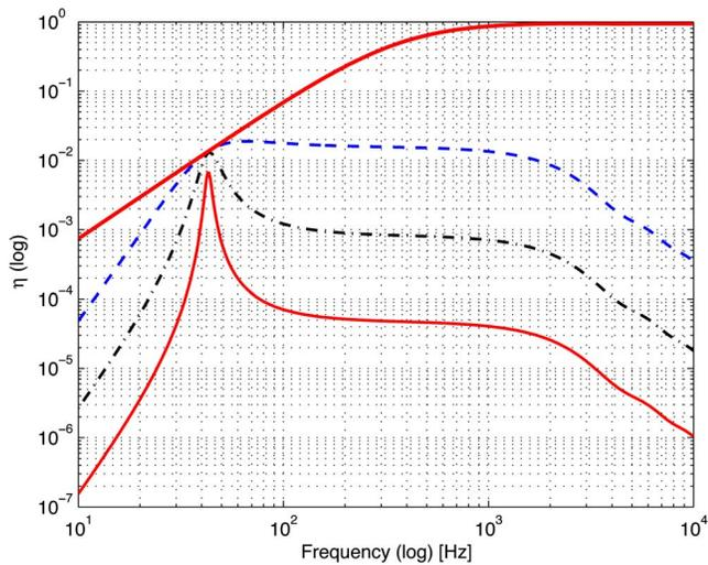
FIG. 3. (Color online) The power efficiency  $\eta$  for the driver MM3c with four  $Bl$  values: low  $Bl=1.2$  (solid), medium  $Bl=5$  (dash-dot), high  $Bl=22$  N/A (dash), and  $\lim_{Bl \rightarrow \infty}$  (thick solid), while all other parameters are kept the same as given in Table II. Note that the efficiency is strongly dependent on  $Bl$  at all frequencies except at resonance, where the efficiency is affected only modestly by  $Bl$ .
