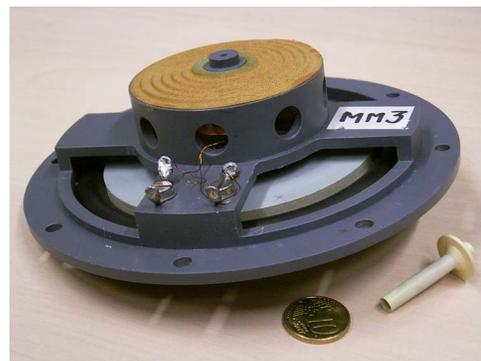
FIG. 5. (Color online) Picture of the prototype driver (MM3c) with a 10 Euro cents coin. At the position where a normal loudspeaker has its heavy and expensive magnet, the prototype driver has an almost empty cavity; only a small moving magnet is necessary, which is shown in the right corner.
