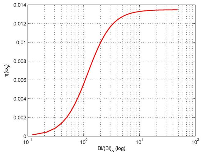
FIG. 4. (Color online) The power efficiency  $\eta(\omega = \omega_0)$  versus the normalized force factor  $Bl/(Bl)_o$  for the driver MM3c, where  $(Bl)_o$  is the optimal force factor given in Eq. (29), in this present case  $(Bl)_o = 1.19$ . The other parameters are given in Table II.
