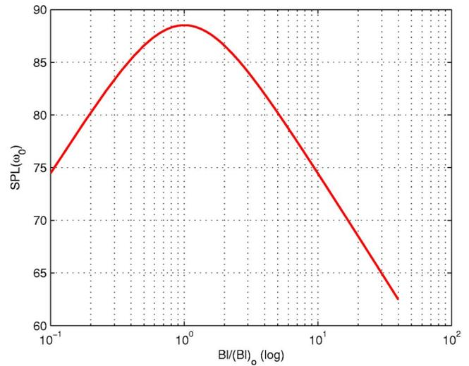
FIG. 2. (Color online) The SPL at the resonance frequency versus the normalized force factor  $Bl/(Bl)_o$  for the driver MM3c, where  $(Bl)_o$  is the optimal force factor given in Eq. (29), in this present case  $(Bl)_o=1.19$ . The other parameters are given in Table II.
