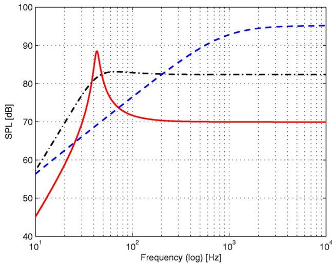
FIG. 1. (Color online) Sound-pressure level (SPL) for the driver MM3c with three  $Bl$  values: low  $Bl=1.2$  (solid), medium  $Bl=5$  (dash-dot), and high  $Bl=22$  N/A (dash), while all other parameters are kept the same as given in Table II, all with 1-W input power and at 1 m distance. At the resonance frequency, the highest SPL is obtained by the low- $Bl$  driver, while the high- $Bl$  driver has at low frequencies—in particular at the resonance frequency—a poor response.
