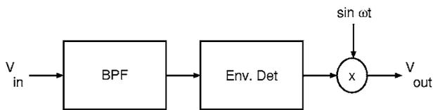
FIG. 6. Frequency mapping scheme. The box labeled “BPF” is a bandpass filter, and “Env. Det.” is an envelope detector. The latter can be a simple rectifier followed by a low-pass filter. The signal  $V_{out}$  is fed (via a power amplifier) to the driver.
