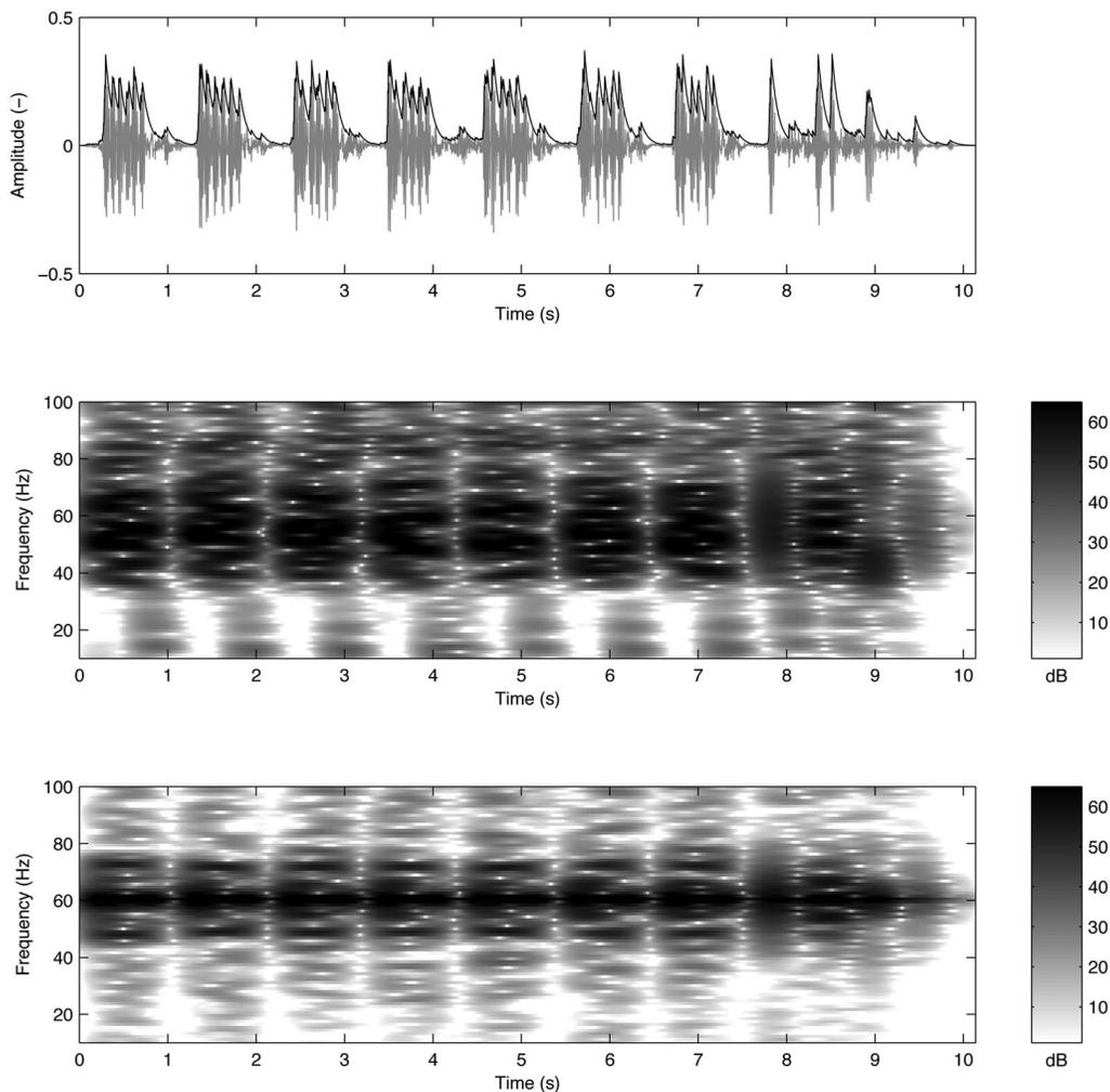
FIG. 7. The signals before and after the frequency-mapping processing of Fig. 6. The upper panel shows the time signal at  $V_{in}$ , and the thin curve the output of the envelope detector. The middle and lower panels show the spectrogram of the input and output signals, respectively.
