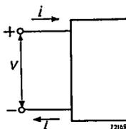
Fig. 2. Positive senses of current and voltage of a terminal pair.
