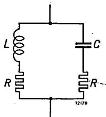
Fig. 3. Two-pole network.
