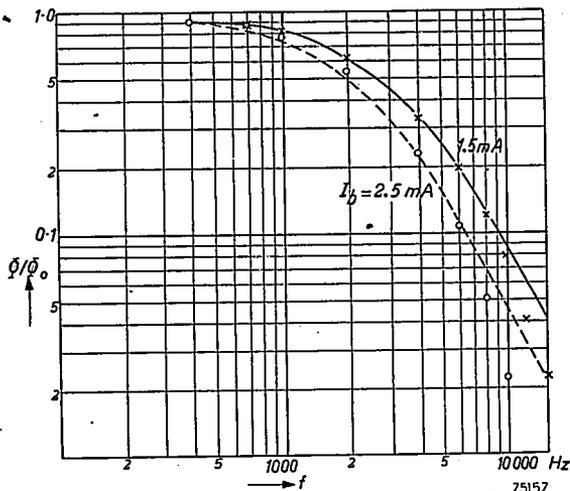
Fig.38. Calculated and measured frequency responses for two values of the biasing current.
