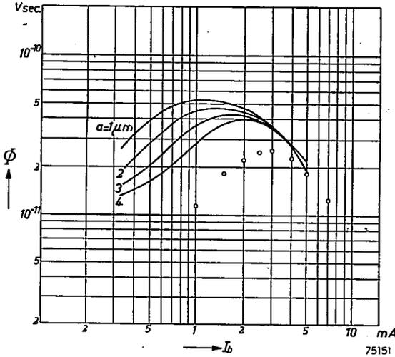
Fig.32. Computed (full curves) and measured flux (circles) as a function of biasing current.
