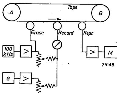
Fig. 29. Schematic diagram of experimental arrangement.
