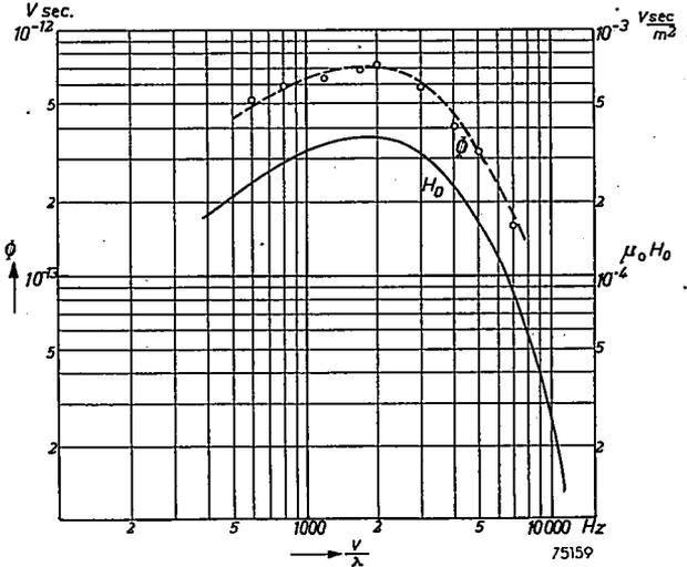
Fig.40. Dependence of printed flux  $\Phi$  and printing field  $H_0$  on wavelength.
