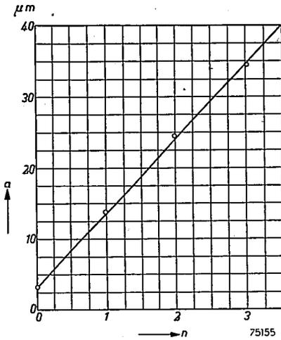
Fig.36. Calculated separation between tape and head against the number of sheets between the two.
